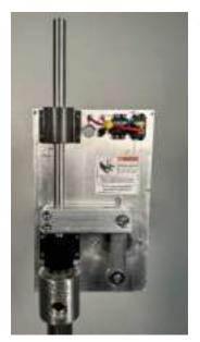
There is a 1/4" of space between the bottom bearing housing and the top of the rod gland when the holes are fully aligned. The rod gland is the topmost exposed component on the pump head.
