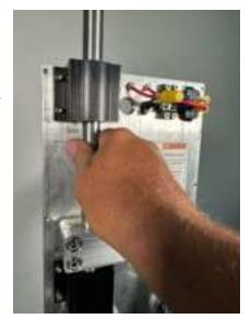
2. If you have passed step 1, tighten the remaining loose screws on both the top and bottom linear bearings, there should be four (4) left to tighten. The unit should be off during this step.
