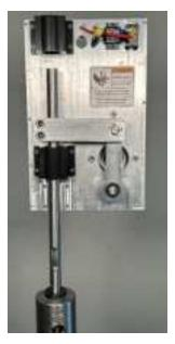
Lower the assembly onto the pump head so that the pump rod and extension are inserted through three (3) openings. As the unit is lowered down, the rods move through the below pieces, in order.
