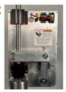
Attach the cover to the LBLD mechanism. Use your 9/64" Allen Wrench for the six (6) 8-32 SS SHCS that attached the cover to the mechanism's mounting plate.
