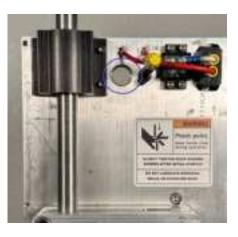
Now that the initial alignment is complete and the power has been connected, we can perform the initial startup. During the initial startup we will verify the alignment and tighten the linear bearings for the break in period.
