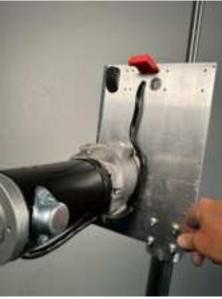
This next step is very important. We will need to make sure the piston is in the correct position. To do this, grab the portion of the 13" rod extension that is sticking out of the top of the unit and pull up. The ideal location for the joint between the standard pump rod and the 13" extension is in the middle of the clevis, as shown in the photo to the right, circled in red. If your rod to pipe ratio is correct, you should need to lift the rod up to get it into the position explained above.
