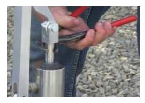
Remove the lever arm, bracket, lever, and clevis (they should still be connected) from the 3/4" stainless rod as shown to the left. These are reverse threads, the direction you screw is the opposite of normal -- turn clockwise to remove, rather than the normal counterclockwise.
