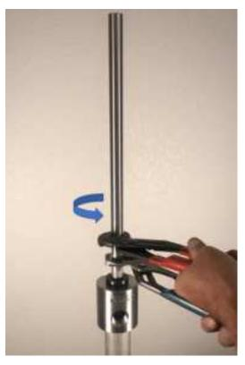
Add the 13" Rod Extension to the top of the existing pump rod. As mentioned above, these are reverse threads so you will go counterclockwise to tighten. Use the two channel locks to tighten as shown to the left.
