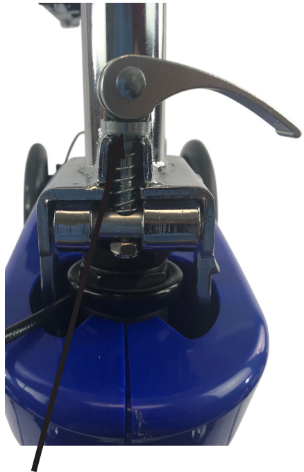
Lever is placed into the “U” slot and clamped down. Steering column is now secure.
