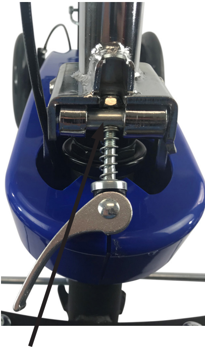
Spring loaded pin. Push to the left to release.
