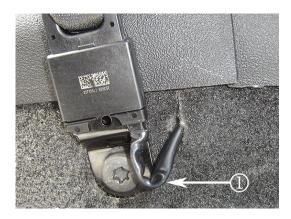
6. Slide the BTS pigtail wire forward to gain additional wire near the sensor as shown allowing the pigtail loop to contact the floor (refer to Figure 8).
