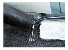
Figure 2 - Outer Wiring Wrap Insulation Breached
