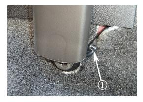
5. Route the new wire pigtail from the BTS to allow extra slack at the previous wire stress area (refer to Figure 7).
