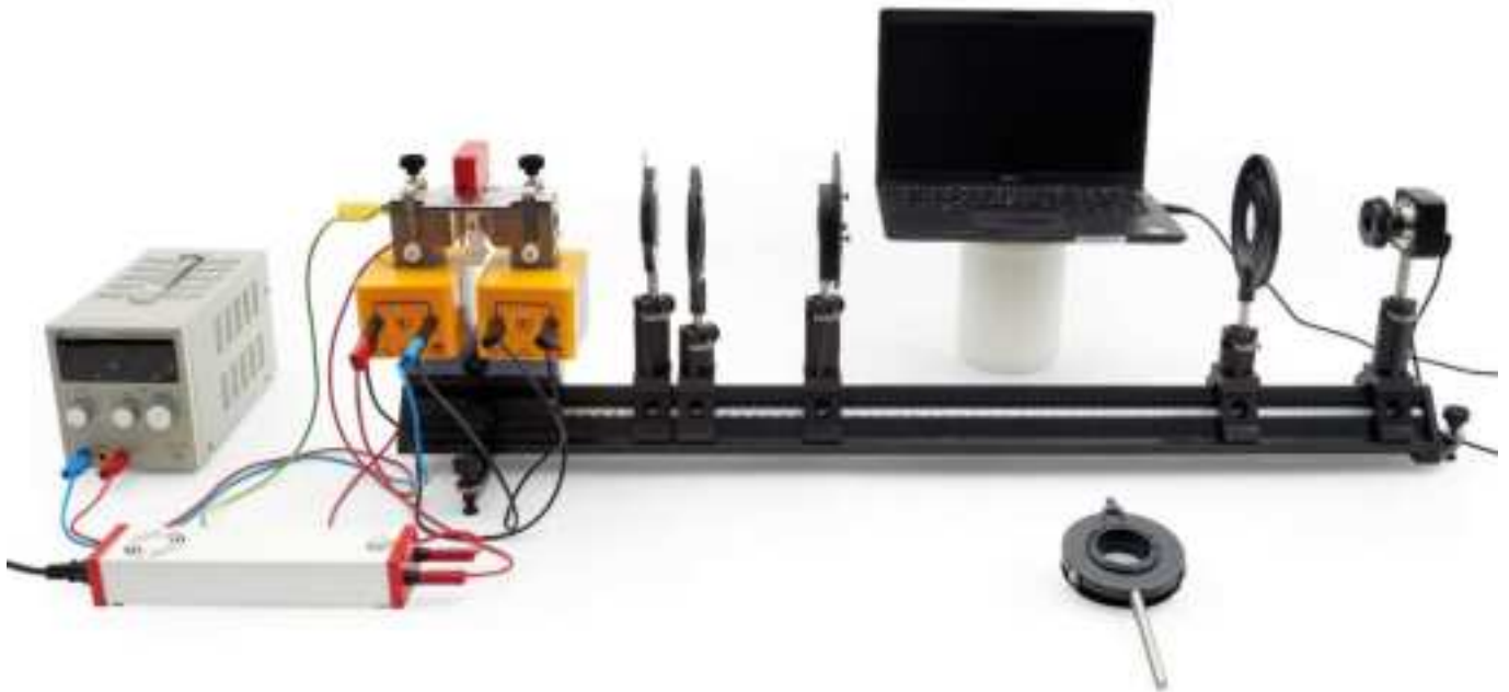
Fig. 1: Experimental setup for the normal Zeeman effect in longitudinal configuration
