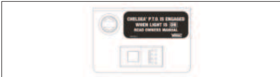
Figure 7 — PTO indicator panel and selector switch
