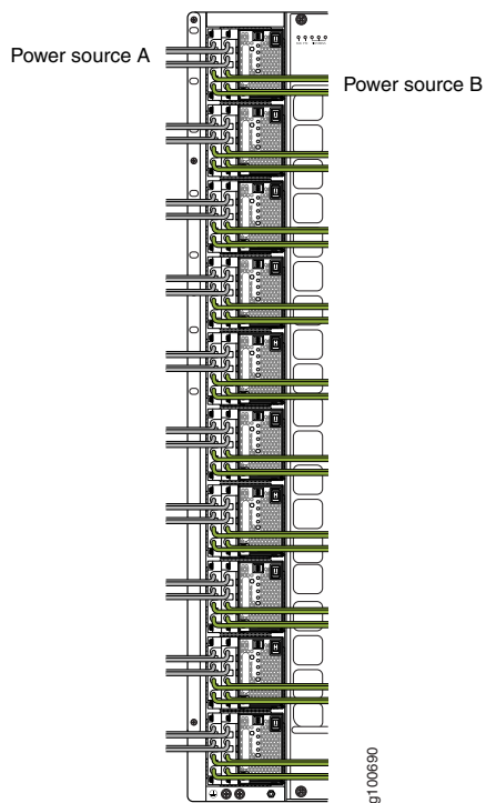
Figure 139: Proper Load Balancing for JNP10K-PWR-DC2 Power Cables on a PTX100016
