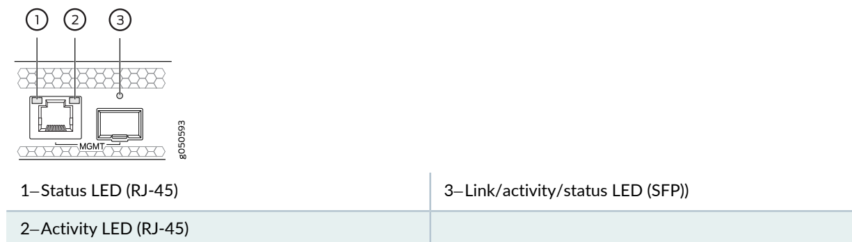
Figure 43: Management Port LEDs on a PTX10016
