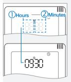
Initially the hour setting is flashing (1).
