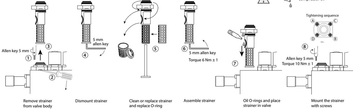
Remove strainer from valve body
