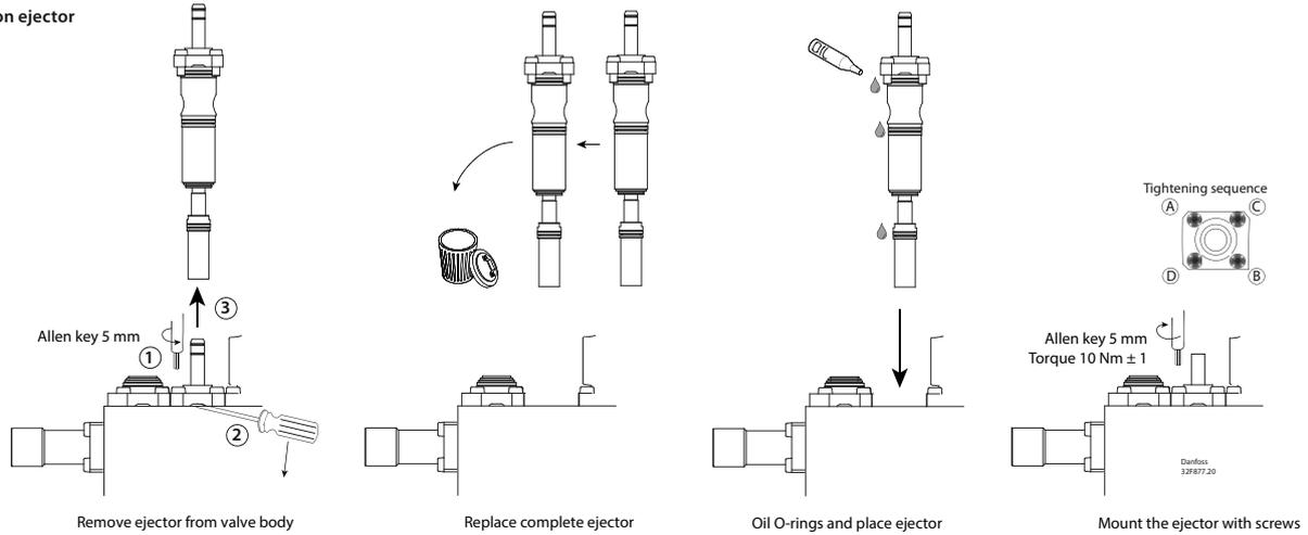
Remove ejector from valve body
