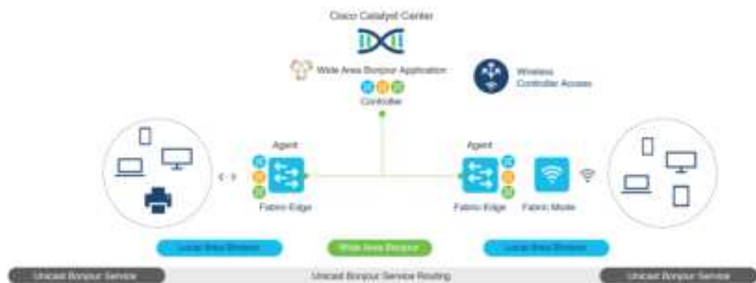
Figure 52: Cisco SD-Access Wired and Wireless Network Design
