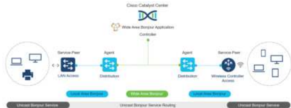
Figure 48: Cisco Wide Area Bonjour Solution Architecture
