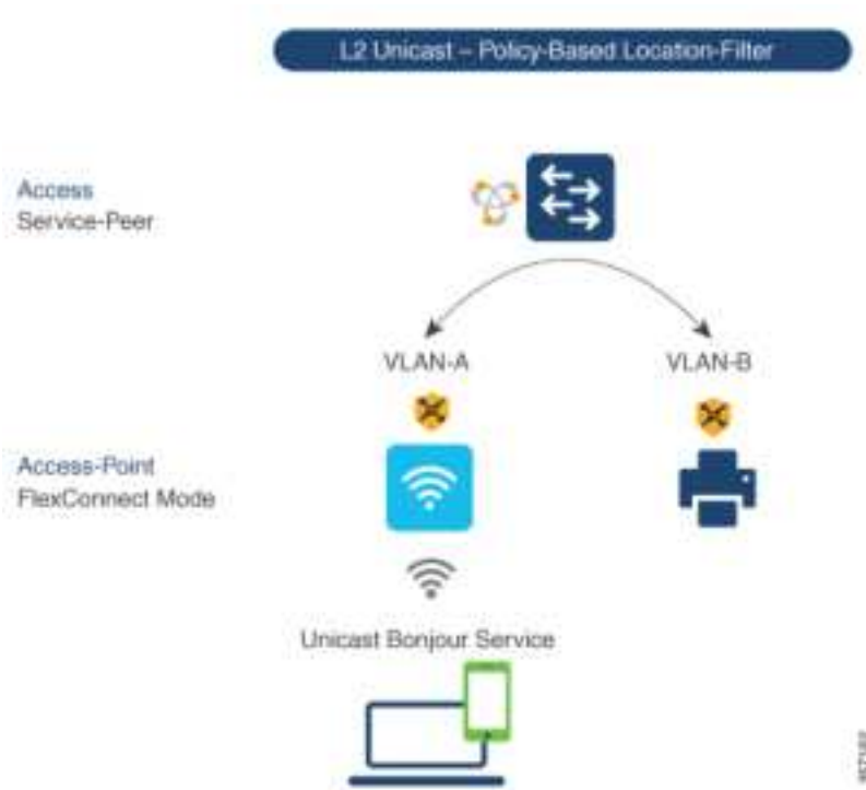
Figure 66: Catalyst Service-Peer mDNS Location-Filter Configuration
