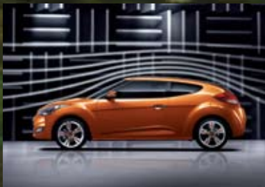
Aerodynamics With its low, coupé profile enhancing the aerodynamics, the reduced drag lowers fuel consumption.
