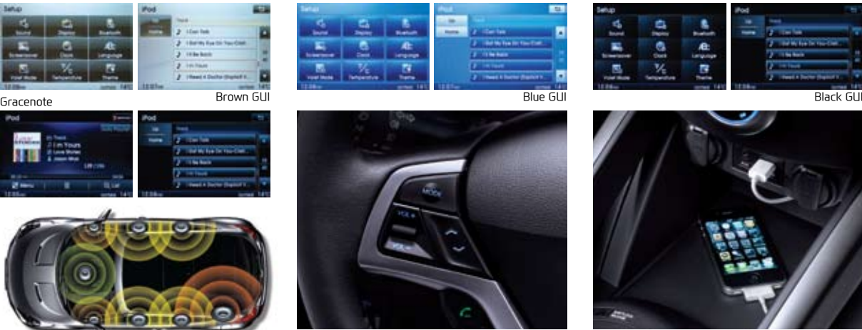
Premium sound system The Mobis premium audio system, features a central speaker, external amplifier and sub woofer.
