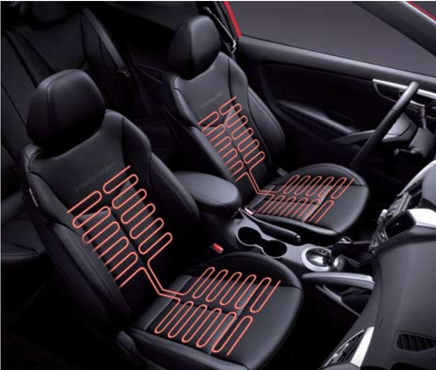
Seat warmers Seat warmers in the driver and passenger seats provide warmth and comfort during cold driving conditions.
