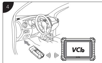
• When the MaxiVCI V200 is properly connected to the vehicle and the tablet, the VCI status button on the bottom bar of the screen will display a green badge at the corner indicating the tablet is ready to start vehicle diagnosis.
