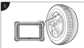
Hold the MaxiCOM MK906 Pro2-TS tablet with its top right corner close to the tire sidewall at the valve stem to activate the TPMS sensor.
