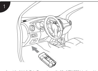
• Insert the Vehicle Data Connector on the MaxiVCI V200 into the vehicle's DLC, which is generally located under the vehicle dashboard.
