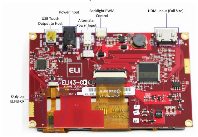
Power may be supplied either via the 2.1mm power jack P2 (center positive) or via the 2-pin terminal block J8
