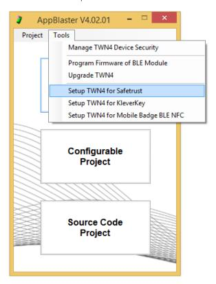
The current firmware running on the BLE Module will be checked in the process and the module will be reprogramed only if the firmware doesn't match the selected setup. The AppBlaster messages window will display the current firmware for the verification. In case reprogramming is necessary, the process may take up to 1 minute.
