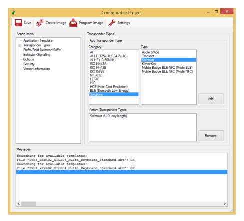
4. Using "Create Image" for compiling a new firmware image and "Program Image" button for loading it on the reader, the process of configuration is finished. The reader now supports "Safetrust" Android and iOS Apps.
