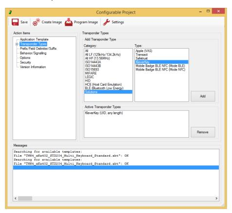
4. Using "Create Image" for compiling a new firmware image and "Program Image" button for loading it on the reader, the process of configuration is finished. The reader now supports "KleverKey" Android and iOS Apps.
