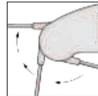
Apply the tip of the probe to the substance, medium or surface to be measured. The sensor is located at the tip of the probe, therefore the minimum depth insertion should be 3 mm.
