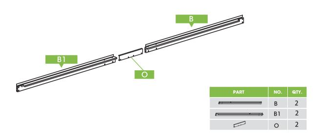
3 Connecting part "B" and part "B1" with 12 screws "U"
