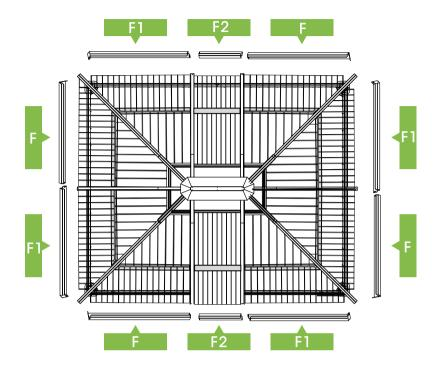
Use 6 parts "X" and 6 screws "U" to fix parts "F" and "F2". Use 4 parts "Y" and 4 screws "U" to fix parts "F" and "F1".
