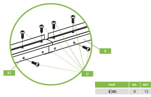
Notice: Before fixing, please make sure all the screw holes are aligned
