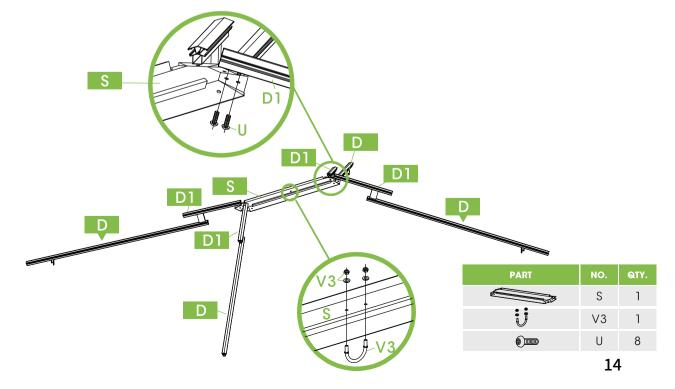
Move the whole roof to the shelf and fix the part "D" with four screws "U".
