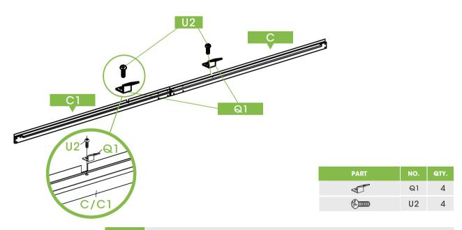
Notice: 1.Before fixing, please make sure all the screw holes are aligned 2. Repeat the above steps to finish conneccng the other part "C" and part "C1".
