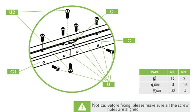
7 Four part "Q1" is fixed at the top with Four screw "U2".
