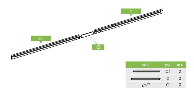
Connecting part "C" and part "C1" with 12 scews "U", fixed with 4 screws "U2".
