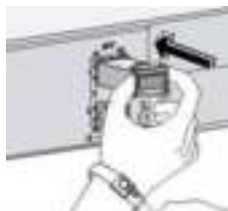
Figure 4-4 SFP module installation
