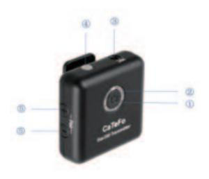
① Power key Long press to turn on or off the transmitter
