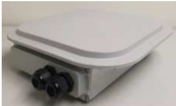
Figure 3: 9502 terminal P/N 3500753-0022 (new antenna)
