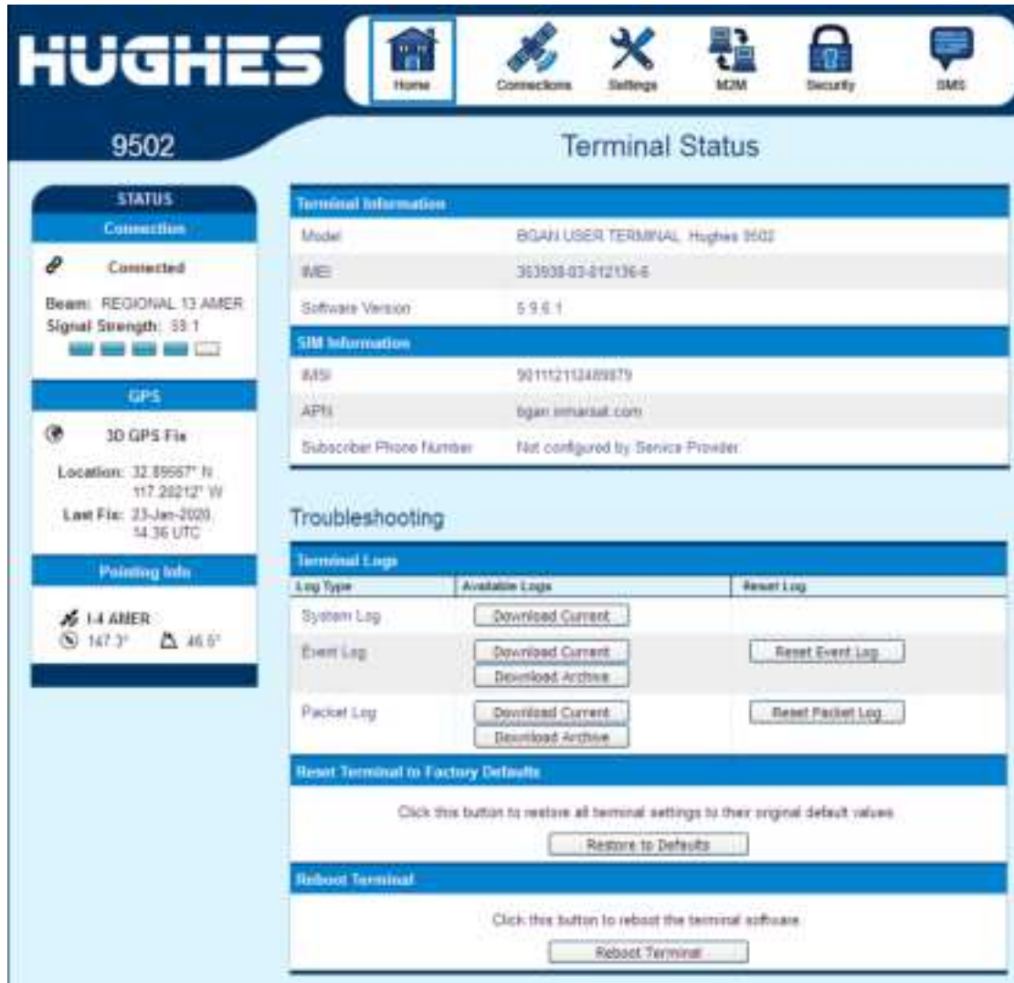
Figure 27: Home page showing pointing information
