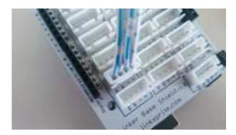
The LK-Temp2 temperature sensor is connected directly to digital port no. 4 of the LinkerKit module, as shown in the illustration. Alternatively, the sensor can also be connected directly to your Raspberry Pi or Arduino. The pin assignment can be seen in the following figure:
