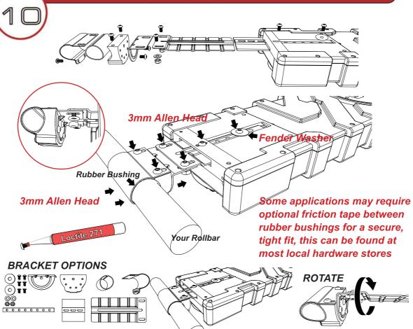
1) Determine the best location on your rollbar for your vehicle, install rubber bushings on the rollbar, ensure there is ample head space 2) Apply supplied Loc-Tight to allen bolt tips, let dry for 20 minutes
