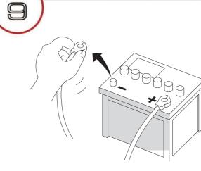
To avoid potential shorts in the electrical system, be sure to disconnect the (-) battery cable before installation. Use this unit with a 12-Volt battery and negative grounding only. Failure to do so may result in a fire or malfunction.
