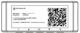
3. Turn on WiFi of your phone and connect: Go to Phone's Settings > WiFi > Select WiFi of the dashcam. After it's connected to the WiFi, it will say 'No Internet Connection' which was normal. Because dash cam WiFi is ONLY for video/photo transfer function, NOT made to broadcast footage over the cloud or internet, please ignore the prompt.
