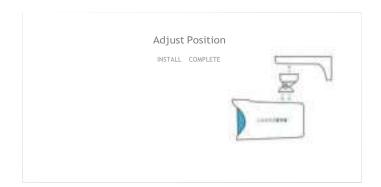
Adjust the camera position and angle as needed to ensure complete coverage, and tighten the screws. Camera installation is now complete.
