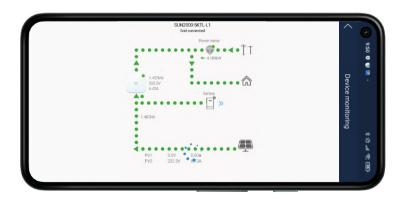
The result should be a diagram in which the photovoltaic power is always positive as well as that of the household. Only the total consumption should be negative if the house is consuming less than the PV system is generating.
