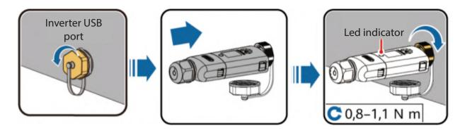
Connect the dongle to the USB port of our inverter as shown in the pictures. After that, the Dongle will start the boot protocol and the LED will start blinking red. When finished, the blinking will be green and it will generate a Wi-Fi access point for 3 minutes.
