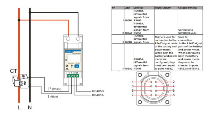
To power the meter, we must connect the phase and neutral of the line we want to measure to pins 3 and 4, respectively. After that, we must establish RS485 communication by connecting pin 24 **(A)** and 25 **(B)** of the meter to pin 3 and 4 of the communications connector of the Huawei inverter respectively. The clamp should be connected according to the following scheme:
