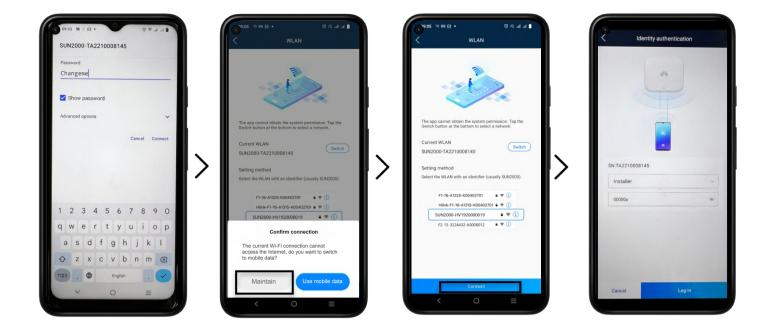
By default, the network SSID will be **SUN2000-(SERIAL NUMBER)** and the password is **Changeme**. Once connected, some devices will show a warning that the network has no internet connection. We will have to press to maintain the connection and then we will press to continue inside the SUN 2000 app. We will be asked for a password for the Installer user, by default it should be 00000a. This will allow us to enter the Home screen.
