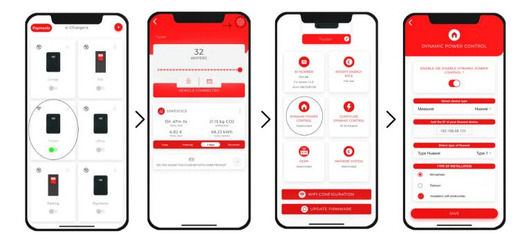
Enter the desired e-Charger and click on the configuration icon at the top right. Enter the DYNAMIC POWER CONTROL section and choose **Huawei** as the slave type and enter the IP address we specified earlier (e.g. 192.168.1.229). After choosing whether our network is single-phase or three-phase and whether it includes photovoltaic installation, we will save the configuration. Trydan will save the configuration and restart to apply these changes.
