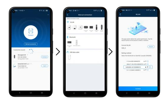
The first thing it shows us is a scanner to configure our inverter. The QR code that can scan is located on the right side of the inverter but in this manual, we will configure the SUN2000 manually. Click on Manual connection and select the image of our inverter.
