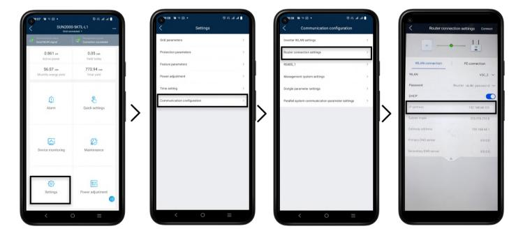
Once we get in the home screen click on **Settings >> Communication settings >> Router connection settings.** We can now see if the router to which it is connected is the same as Trydan or if it needs to be configured. If it is configured, we should note down the IP it occupies in our network for further configuration of Trydan.
