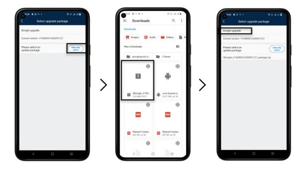
Click on **Dongle Update** and wait for the process to finish following the instructions on the screen. This process should not modify the Wi-Fi configuration of the inverter, but it is advisable to check it later by entering the inverter configuration. Once this process is done, the communication between the inverter and Trydan will be re-established.
