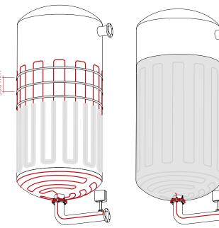
Fastening with tension strap or with aluminium adhesive tape.
