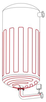
Basically, the heating cables are laid in a meandering manner on vessels and on surfaces. Wrap the vessels with the heating cable only if the project planning explicity prescribes it.
