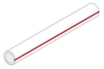
Normally the heating cable is laid streched out along the pipe. Lay heating cables in a spiral pattern only if the projects planning explicity calls for it.
