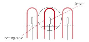
The temperature sensor must be installed centrally between the heating cables. Care must be taken to ensure the best possible contact between the sensor and the surface.
