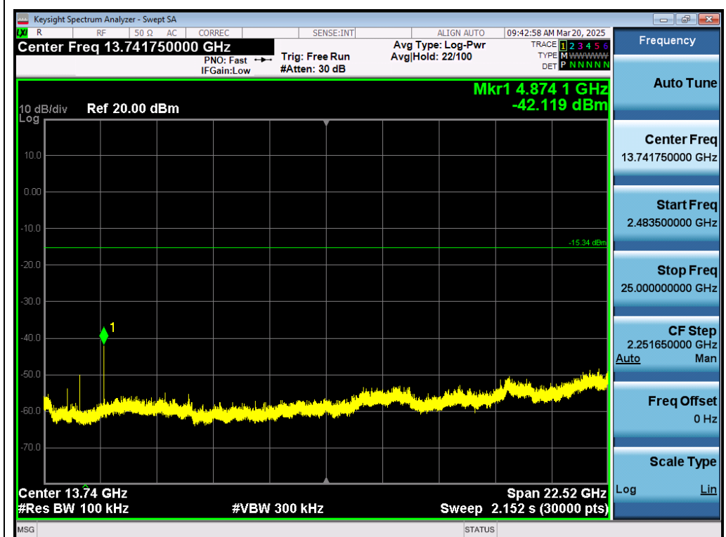
Test_Graph_802.11b_ANT1_2437_1Mbps_Higher Band Emissions
