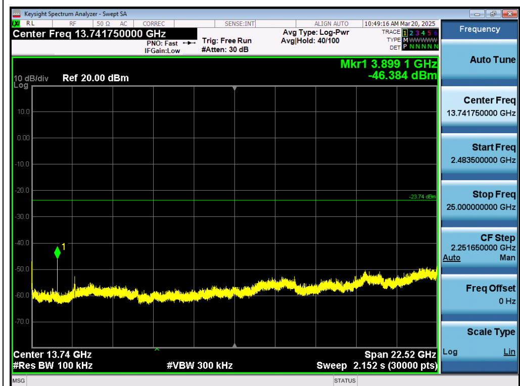
Test_Graph_802.11ax40_ANT1_2437_MCS0_Higher Band Emissions
