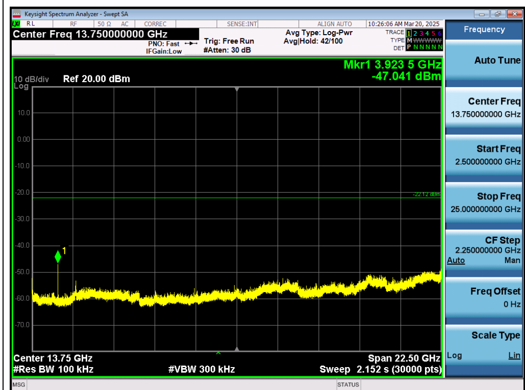
Test_Graph_802.11n40_ANT1_2452_MCS0_Higher Band Emissions
