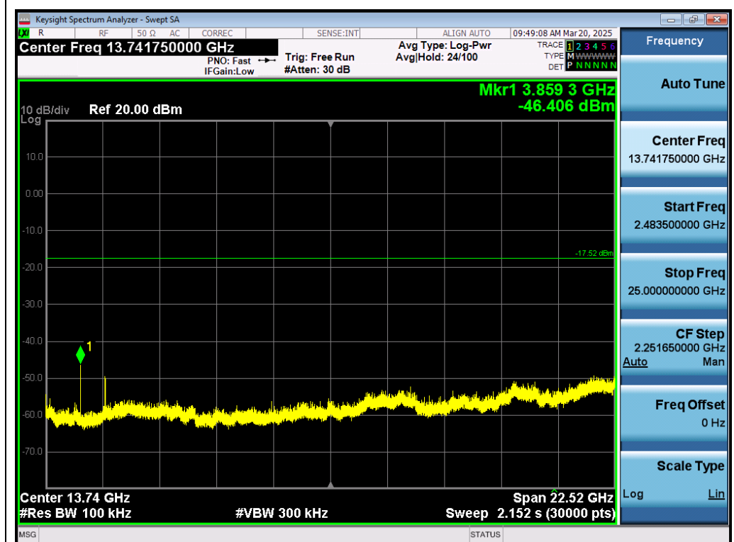
Test_Graph_802.11g_ANT1_2412_6Mbps_Higher Band Emissions
