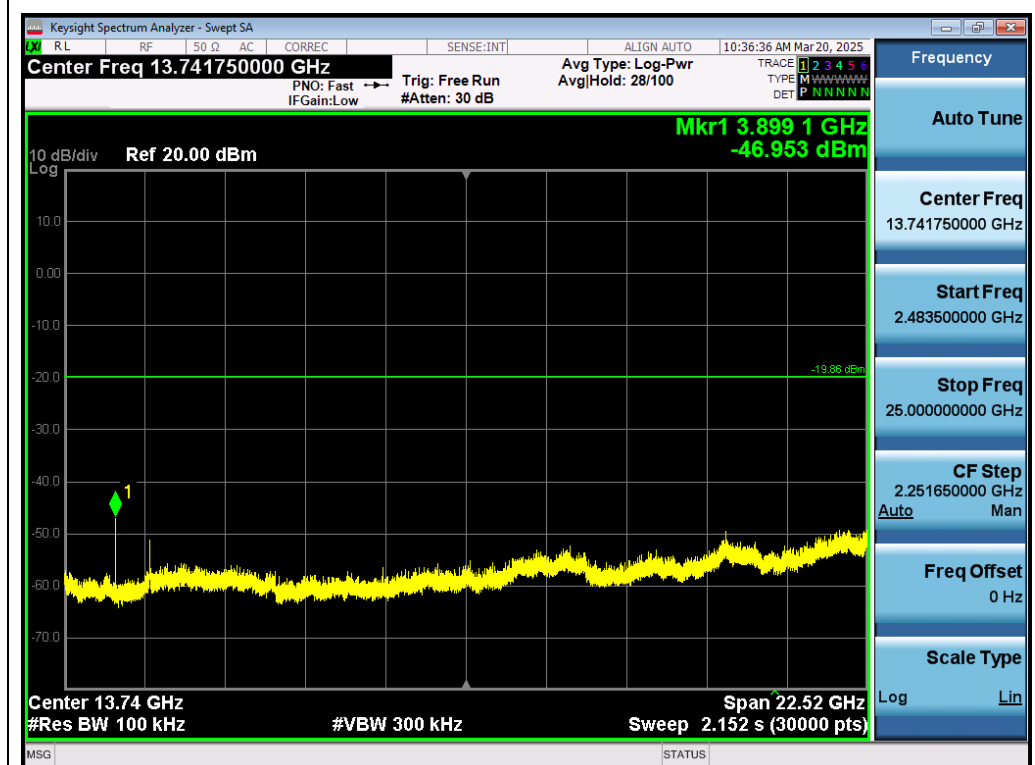
Test_Graph_802.11ax20_ANT1_2437_MCS0_Higher Band Emissions
