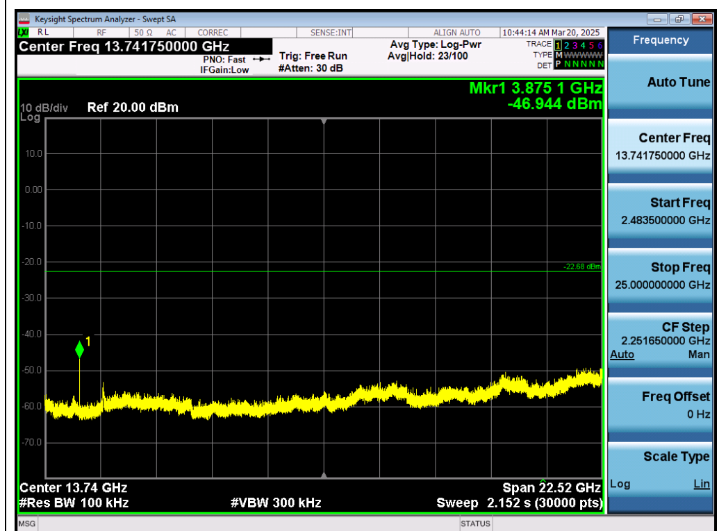
Test_Graph_802.11ax40_ANT1_2422_MCS0_Higher Band Emissions
