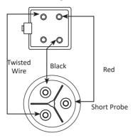
**Ohm Water Level Probe and Wiring Harness**
