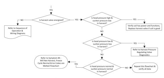
Single Evaporator Systems with Dual Harvest Valves: If one Harvest Vavle is open and the other is restricted / stuck closed you may have normal harvest pressures. Look for ice not melting on one side of the evaporator.
