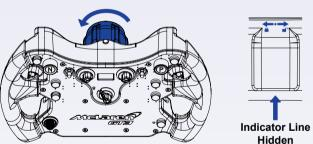
For attachment to a Podium Wheel Base DD, ensure that the locking nut is touching the rubber gasket but < not compressing it. Turn the SQRA screw nut in the open lock direction until the indicator line is completely exposed, then slide the steering wheel onto the wheel base shaft. Once the steering wheel is seated at the mechanical limit, turn the SQRA screw nut in the closed lock direction until the indicator line is completely covered.
