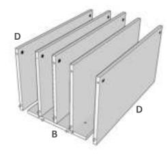
Step 5: Finish unit by adding end panels (A). Lock cam pins in by turning cam locks 90 degrees
