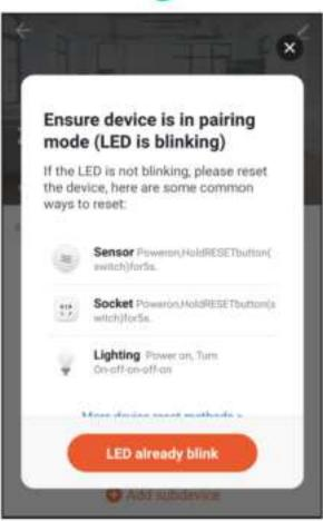
• Remove the insulation sheet and press the reset button for 5 seconds, till the blue LED blink, then click "LED already blink" on the app.
