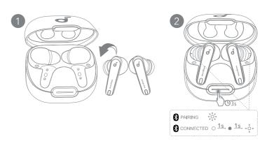
To manually enter Bluetooth pairing mode, place the earbuds in the charging case and leave the case open. Press and hold the charging case button all the way down for 3 seconds until the LED indicators flash white rapidly.
