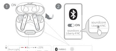
Open the charging case, the earbuds will automatically power on and enter Bluetooth pairing mode. Select "soundcore Liberty 4 NC" from your device's Bluetooth list when connecting for the first time.
