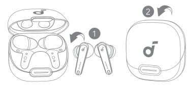
To power off, return the earbuds to the charging case and close it. The earbuds will automatically power off after 30 minutes if they are not connected. The duration can be set in the soundcore app.
