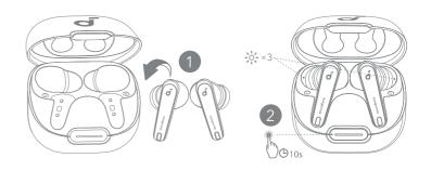
Reset if the earbuds have issues pairing with each other or with other devices. Delete the pairing history from your Bluetooth device first. Place the earbuds in the charging case and leave the case open. Press and hold the charging case button for 10 seconds until the LED indicators flash white rapidly three times.
