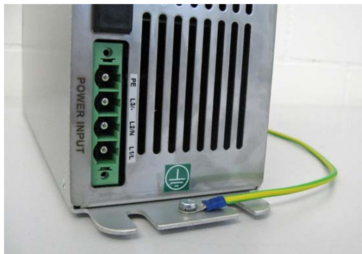
Figure 26: AC power input and protective earth of LPC-4000 controller
