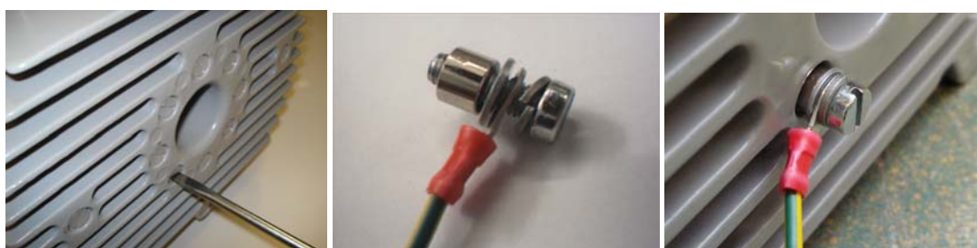
Figure 31: Attachment of a protective earth wire to the backside of the motor
