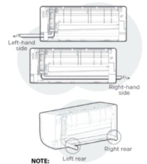
Based on the position of the wall hole relative to the mounting plate, choose the side from which the piping will exit the unit. You have four options for the exit direction of the piping.
