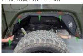
Attach the rubber strip to the fender flare. Align it with the factory installation holes of the vehicle.
