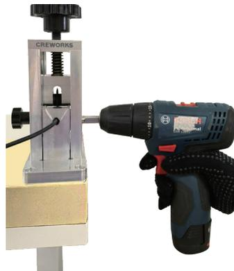
If your wire's insulation is not removed, stop use, raise the blade, remove your wire, and then further lower the blade before beginning again.
