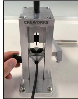
3. Insert your wire and then lower the blade by turning its adjustment knob clockwise until you feel the blade touch your wire.
