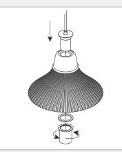
5. Adjust the length of the lighting cable using the grub screw on the end of the cable.
