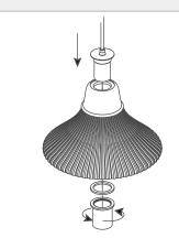
5. Adjust the length of the lighting cable using the grub screw on the end of the cable.
