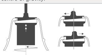
6. Hook the adjusted cable through the ceiling rose cover and slide into the centre of the pre-mounted plate.
