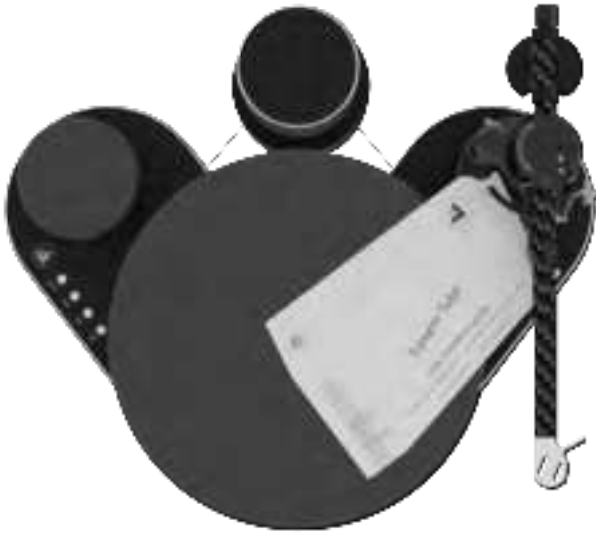
Pic. 13: Positioning the alignment gauge
