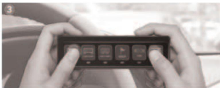
After configuring all buttons, long-press any two buttons simultaneously for 3s again. The yellow indicator will flash once and turn off, confirming the settings are complete.
