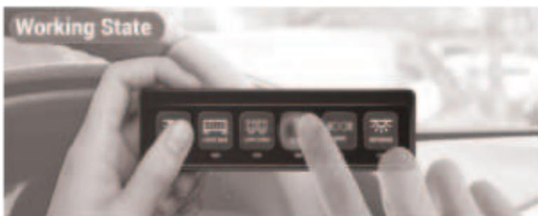
In the standby state, press any button, and the **YELLOW** indicator lights up, indicating that it enters the working state.
