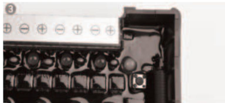
When the pairing button indicator flashes 3 times, now the pairing is successful.
