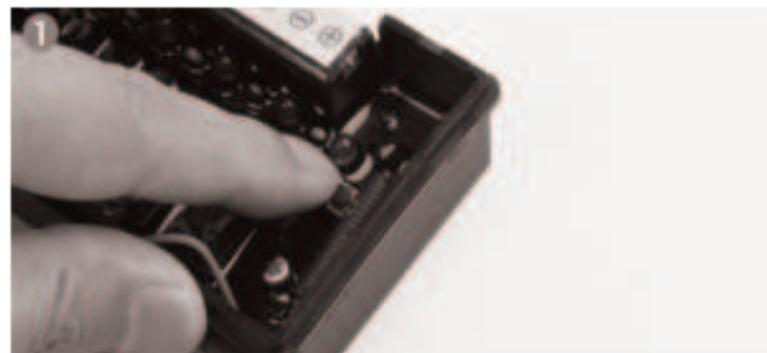
Press the pairing button on the control box.
