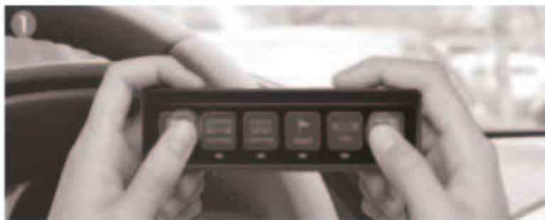
Power on the panel. Long-press any two buttons simultaneously for 3s until the white backlight turns off and Yellow Indicators light up/start flashing, now you've entered Control Mode Setting.
