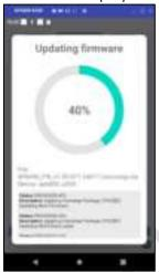
5. When the firmware update completes, the log displays "The firmware updating process is done," and shows the FW version. Select OK to return to the main screen to complete the ICC262R firmware update.
