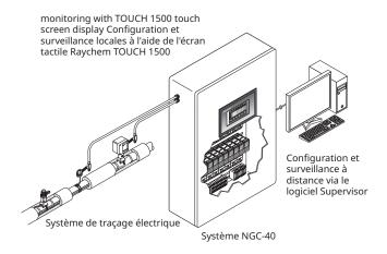
The Raychem NGC-40 is a multipoint electronic control system with a unique single point controller architecture for heat-tracing used in process temperature maintenance and freeze protection applications. By taking advantage of innovative modular packaging techniques, the NGC-40 control system provides configuration and component flexibility so that it may be optimized for a customer's specific needs.
