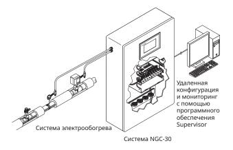
The Raychem NGC-30 is a multi-circuit electronic control system for heat-tracing used in process-temperature maintenance and freeze-protection applications. The NGC-30 Controller can accommodate temperature inputs from a variety of sources: hard-wired to the panel mounted CRM(S) modules or from Remote Monitoring Modules (RMM3).
