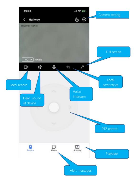
Depending on the hardware capabilities, the functions displayed on the app may be different. If it isn't a PTZ camera, there isn't a PTZ control panel.
