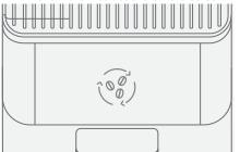
02. Remove Bean Hopper: Unlock hopper knob and press down on the side removal button.
