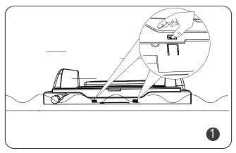
There are two small fasteners on the top of the docking station, and you can push them to remove the main part from the hook.
