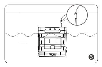
Insert the included extended charging line to the socket on the line of the station.
