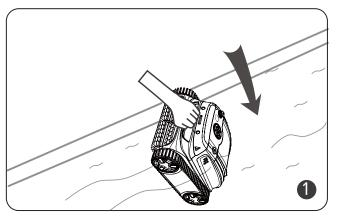
Hold the handle of the cleaner, and emerge it into pool water vertically.
