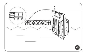
Place the main body of the station onto the hook.
