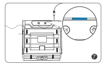
Plug the adaptor into a power supply, and the LED indicators turn solid blue.
