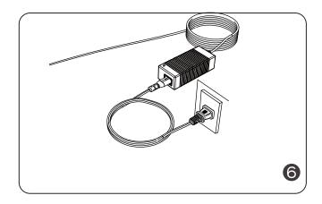
Stretch out the charging line and plug the adaptor into a power outlet that should be at least 3.5m(11.5ft) away from the pool.
