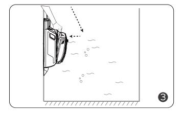
Put the cleaner onto the docking station carefully or put it into the pool and call it to the docking station.
