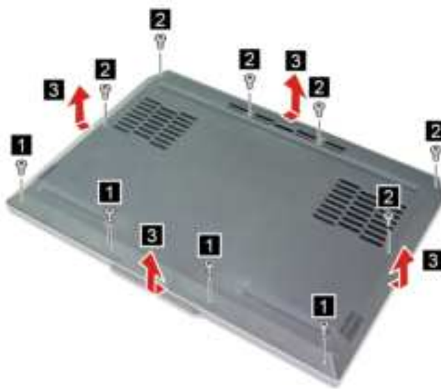
Figure 5. Remove ten screws and the lower case
