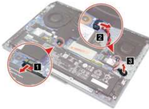
Figure 13. Disconnect the battery pack cable, disconnect the CMOS battery cable, and remove the CMOS battery
