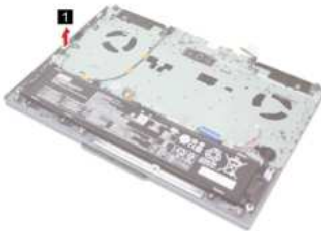
Figure 24. Remove the Type-C bracket
