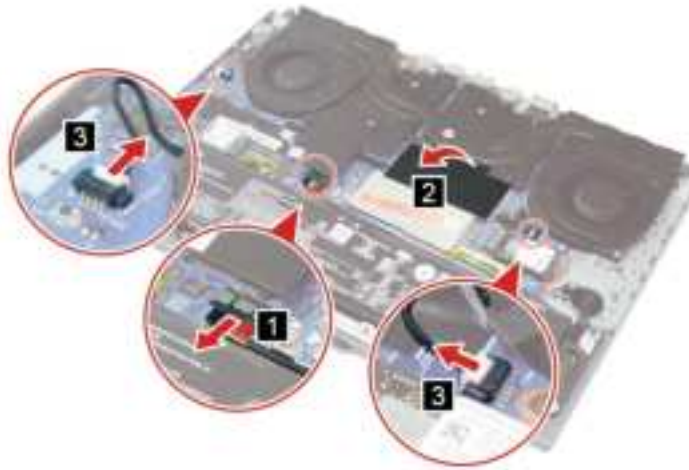
Figure 19. Disconnect the battery pack cable, peel back the mylar, and disconnect the fan cables
