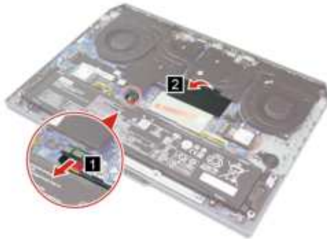
Figure 14. Disconnect the battery pack cable and peel back the mylar
