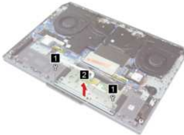
Figure 7. Remove two screws and remove the touchpad bracket
