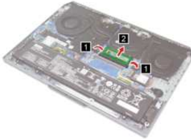
Figure 16. Open the latches and remove the memory module
