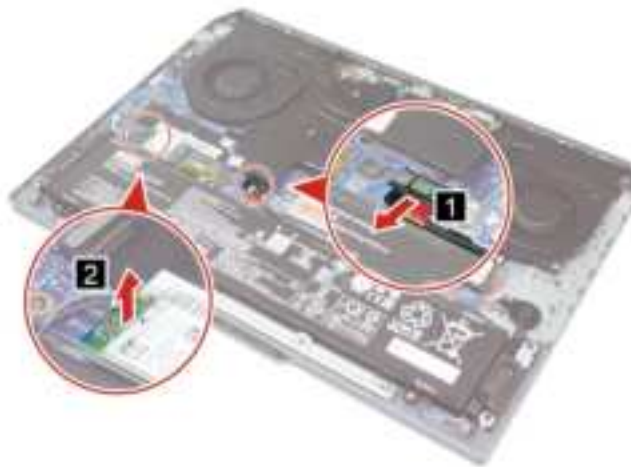
Figure 10. Disconnect the battery pack cable and remove the Wi-Fi mylar
