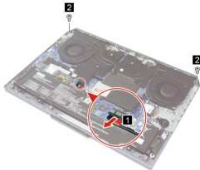
Figure 17. Disconnect the battery pack cable and remove two screws
