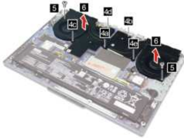
Figure 20. Loosen five heat sink screws, remove two fan screws, and remove the thermal module
