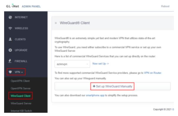
After copy the JSON or Plain Text from your server, you can paste it in the Configuration and then click **Add** to finish the WireGuard Client setup.
