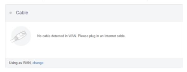
Plug the Ethernet cable into the WAN port of the router. The information of your connection will be shown on the Cable section. DHCP is the default protocol. You can click Modify to change the protocol.
