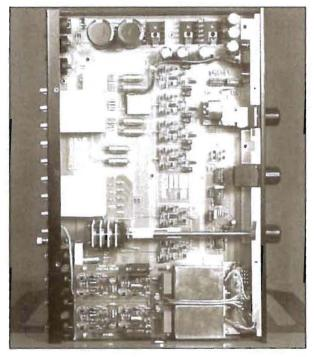
Dense Packaging: It is quite remarkable what the exquisite Bryston preamplifier combines in electronics and manifold connection options within the smallest possible space. The compact dimensions are possible because of the external power transformer.
