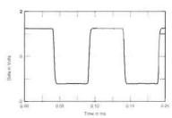
Fig.2 Bryston 9B-THX, small-signal 10kHz squarewave into 8 ohms.
