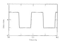
Fig. 18 Bryston 7B-ST, small-signal 10kHz squarewave into 8 ohms.
