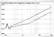
Fig.3 Bryston B-60R, crosstalk, L-R (top) and R-L (bottom) (10dB/vertical div.)
