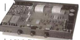
Left in the Picture: The Encapsulated Transformers in the **BP 25 Preamplifier**
