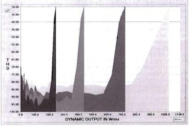
Fig.8 Bryston 9B-THX, distortion (%) vs 1kHz burst output power into 8 ohms (black trace), 4 ohms (red), 2 ohms (blue), and 1 ohm (green).
