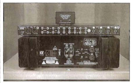
Hook-Up Marvel: The Bryston preamplifier provides balanced inputs as well as outputs. Also the power amplifier is preferably connected in this professional manner.
