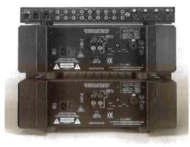
connection. The outputs are five way binding posts with gold plated contacts. Between them is the isolation ridge which prevents the short-circuit by bare wire. Nice touch. The power cord is three-prong.
