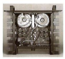
heavy-duty PCB connectors. The power transistors are hand-matched, each driver - output pair is handled as a composite output element in the "Quad-complementary" configuration.
