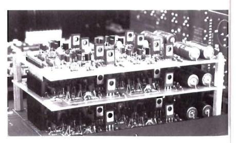
Double Decker. All six of the SP1 outputs are driven by discretely built, symmetrical, stages
