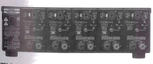
With the balanced inputs, when desired, the volume control can be disabled, then they play (no longer conforming to THX) 6 dB louder. The small jacks on the left side are for remote control operation.
