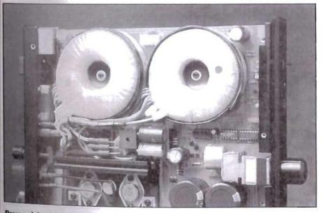
Prerequisite for the Shallow Construction Height: Bryston Uses Two Flat Toroidal Transformers. The Encapsulated Motor Potentiometer is from Alps.
