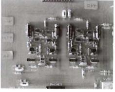
the large Bryston power amplifiers. Thanks to the metal chassis two power transistors are used per channel in order to be able to deliver almost 110 watts continuous operation into four ohms. Carefully thought out signal paths, high quality potentiometers and switches, special German made electrolytic capacitors -
