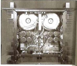
The secret of the ultra-stable bass reproduction of the Bryston power amplifier revealed. Prodigious filter capacity and two massive toroidal transformers. Noteworthy is the service friendly and also thermally thought out construction, which makes it clear why Brystonia able to offer a 20 year warranty.
