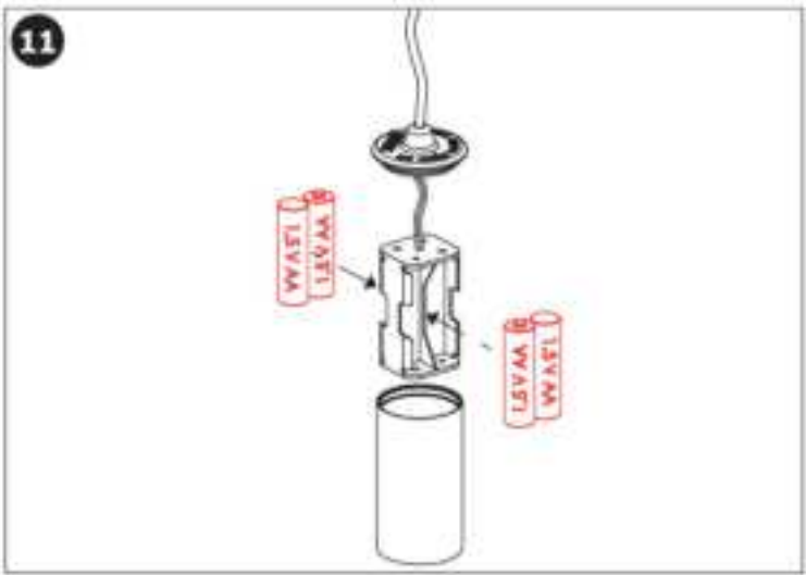
Insert 4 x AA batteries into battery housing ensuring correct polarity
