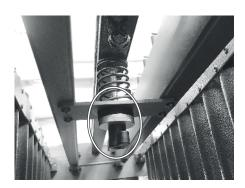
Place the damper beam (21) with the spring on the mounting plate provided between bar 2 (13) and bar 3 (14). Align the connecting arms (22) so that they point towards the semitone resonator (16, open tubes).
