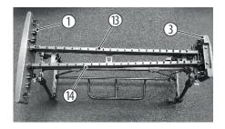
Place the pre-assembled unit consisting of bar 2 (13) and bar 3 (14) in the mounts provided on the upper parts (1, 3).
