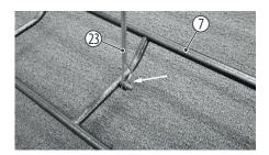
Hook the pedal pull rod (23) into the mount on the pedal rod (7) as shown.
