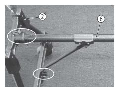
Insert the centre rod (6) into the slot of the wide base (2). Pay attention to the markings (red dots) on the centre rod and the mount.
