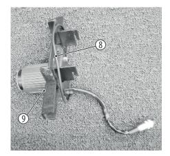
Hang the drive belt (8) on the motor unit (9) as shown.
