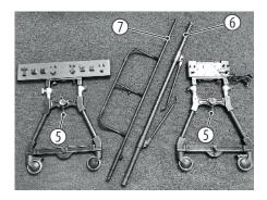
Pull the cotter pin (5) out of the slot for the centre rod (6) of the wide and narrow base.
