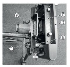
Hook in the motor unit (9) with the drive belt on the control unit (10) of the narrow upper part (3) as shown.
