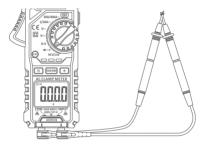
3. Turn the rotary dial to the "V~" setting. The screen will display "♠C" indicating that the measurement function is AC voltage.
