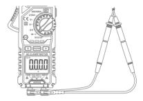
3. Turn the rotary dial to the " $\Omega H$ " setting. The screen will display " $\Omega$ " indicating that the measurement function is resistance.
