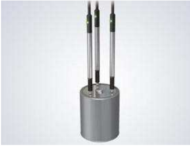
Battery flatness check
